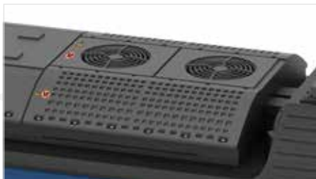
Correct implementation of air conditioning units on the roof
