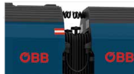
Reproduction of the connection lines between individual coaches
